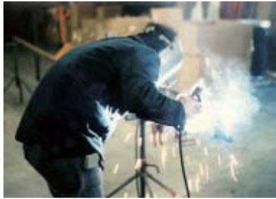
The oxy-acetylene flame is made by mixing oxygen and acetylene gases in a special welding torch or blowpipe, producing, when burned, a heat of 6,300 degrees, which is more than twice the melting temperature of the common metals. This flame, while being of intense heat, is of very small size.
