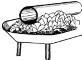
Image Figure 4.—A Gaspipe Annealing Oven
