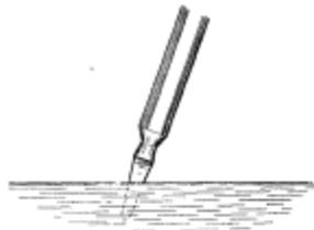
Image Figure 6.—Cooling the Tool for Tempering
